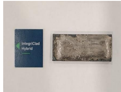
IntegriClad™ welding rope, Ni-based bonding powder layer, and deposited overlay sample prior to metallographic preparation.
