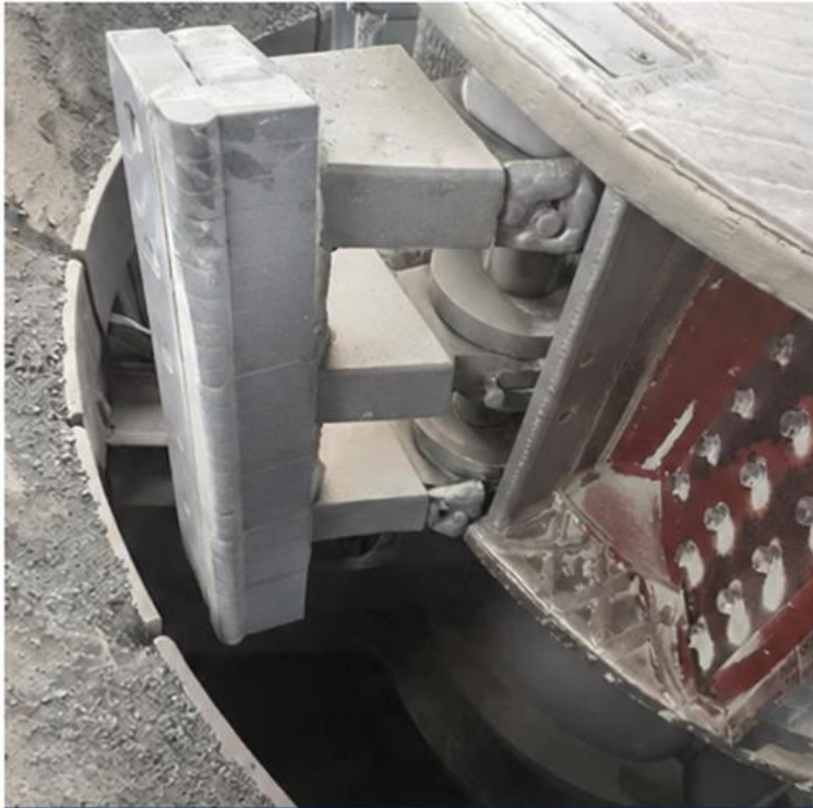
VSI crusher equipped with tungsten carbide crusher blades.
